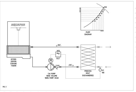
When the thermal load is diminishing, the VFD will reduce the pump speed and eventually stops and remains in a standby mode.
