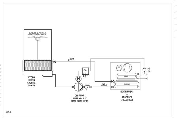
The cooling tower pumps can be controlled by the chiller cold water temperature. The flow switch, mostly common in chiller systems to protect the compressor from a lack of cooling water, should be trigger if flow is < 50%.
