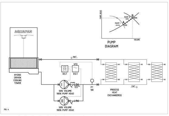
The system starts with pump I in operation on operation point -A-.
