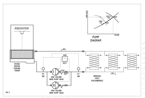
This is the most economic way to operate AQUAFAN cooling towers. Both pumps are controlled to hold the CWT over the whole range at minimum energy consumption.
