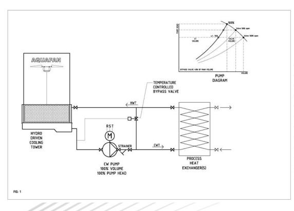
The head pressure goes down and the water is divided between the cooling tower and the bypass valve.
