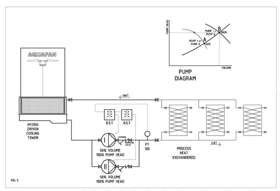
In this set up the basic load pump I covers also ca. 70% of the annual operation while pump II regulates the water flow to keep a constant CWT.
