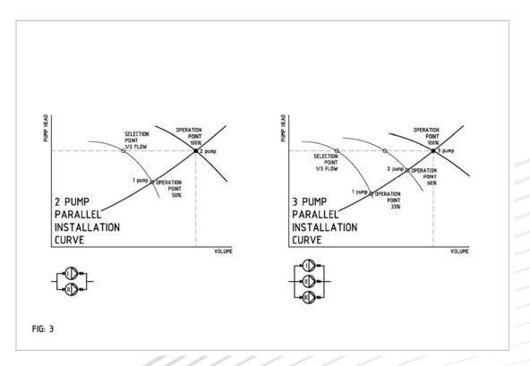
More then 3 pumps in a system loop is not advised as the last pump has hardly any contribution to achieve the max. operation point, unless it is desired in terms operational variety or as spare pump.
